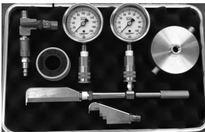
**#804 Shortie Test Kit Ultra:** Our best compact test kit. Includes the #107A ultra-light quick disconnect pitot tube with the ultra-thin straight blade and a spare #112 ultra-thin notched blade. For the gauges, 2 of the #204 Ashcroft model 1009AW flutterguard gauges (any psi) with NIST calibration certificates. We complete this kit with the #301 brass hydrant test cap, #404 double ball valve quick disconnect bleeder and Plano #903 deluxe case. Reg. \$494.65 **\$410.00**
