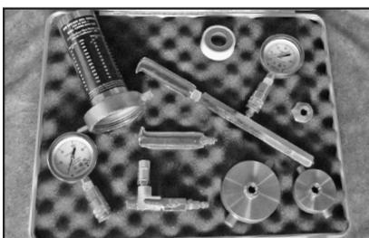
**#805 All Purpose Test Kit:** Includes all of our most popular items. #101 quick disconnect pitot tube w/ #108 spare blade, 2 of the #201 new NEMCO Custom Model liquid filled gauge (2 1/2" Dial, Model BRNEM), #501 inspector's hydrant flow nozzle, #404 double ball valve quick disconnect bleeder, #301 brass hydrant test cap, #303 brass hose cap, #304 brass faucet test cap and #904 Plano large deluxe carry case. Reg. \$532.40 **\$445.00**
