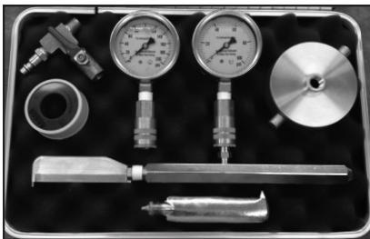
**#803 Shortie Test Kit Deluxe:** An upgrade for the frequent user: #101A quick disconnect pitot tube with ultra-thin straight blade, plus a #108 spare blade. For the gauges, 2 of the #202 (1% full scale accuracy liquid filled model - 2 1/2" dial any psi). The #402 single ball valve quick disconnect bleeder and #301 brass hydrant test cap along with the #903 plano deluxe case finish this package. Reg. \$405.65 **\$335.00**
